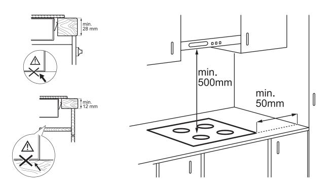
$<sup>^{*}</sup>$ The clearance must meet or exceed the minimum recommended for both the rangehood and cooktop. Refer to the rangehood installation manual.
