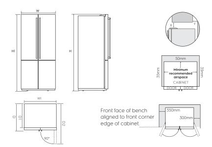
If you have a cupboard above the refrigerator with a rear gap of less than 100 mm (Y), recommended minimum clearance at the top of the refrigerator increases from 30mm to 70mm (X).
