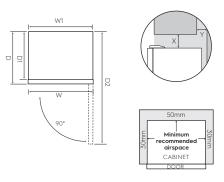
If you have a cupboard above the refrigerator with a rear gap of less than 100 mm (Y), recommended clearance at the top of the refrigerator increases from 50mm to 90mm (X) minimum.
