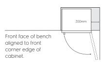
When positioned in a corner area, spacing of at least 350mm on the hinge side will allow the doors to open enough to enable the removal of bins and shelves.
