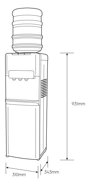
Please note! Dimensions to be used as a guide only. All customers MUST refer to the user manual supplied with the product for detailed installation instructions. © 2021 Electrolux S.E.A PTE. LTD. E\_DIM\_EQACFISXSG\_Sep20
