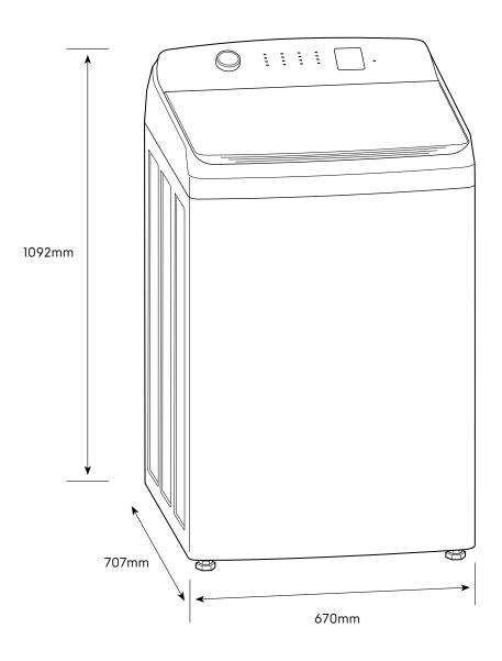
Please note! Dimensions to be used as a guide only. All customers MUST refer to the user manual supplied with the product for detailed installation instructions. © 2022 Electrolux S.E.A PTE. LTD. E\_DIM\_EWTI574M7WA(ARABIC)\_Jan22
