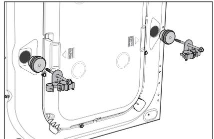
**!** Transit bolts must be removed before using the appliance.
