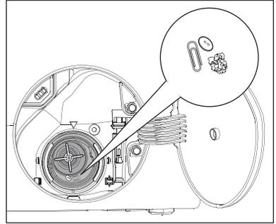
6. Make sure that the impeller of the pump can turn. If this does not occur, contact the service centre.
