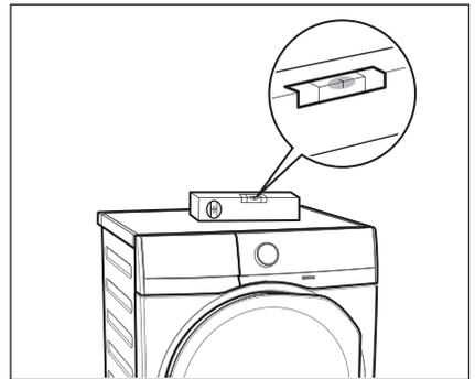
If you do not have a spirit level, as a guide use the edge of a door frame, cupboard or bench to check that the Washer-Dryer is leveled.
