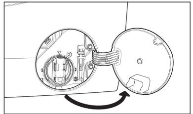
2. Place a suitable water container below the recess of the drain pump to collect the water that flows out.
