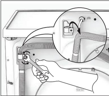
4. Put the end of the drain and inlet hose in a container. Let the water flow out of the hoses.
