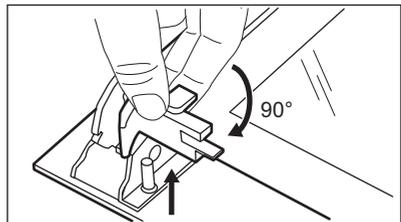
**Step 6** First lift carefully and then remove the glass panel.
