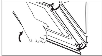
**Step 4** Put the door on a soft cloth on a stable surface and release the locking system to remove the internal glass panel.
