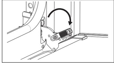
**Step 3** Close the oven door halfway to the first opening position. Then lift and pull to remove the door from its seat.
