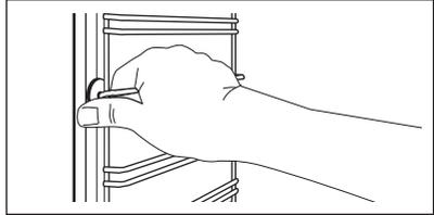
**Step 3** Pull the rear end of the shelf support away from the side wall and remove it.
