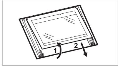
**Step 7** Clean the glass panels with water and soap. Dry the glass panels carefully. Do not clean the glass panels in the dishwasher.
