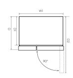
When positioned in a corner area, spacing of at least 427mm on the right hinge side and 349mm on the left hinge side will allow the doors to open enough to enable the removal of bins and shelves.
